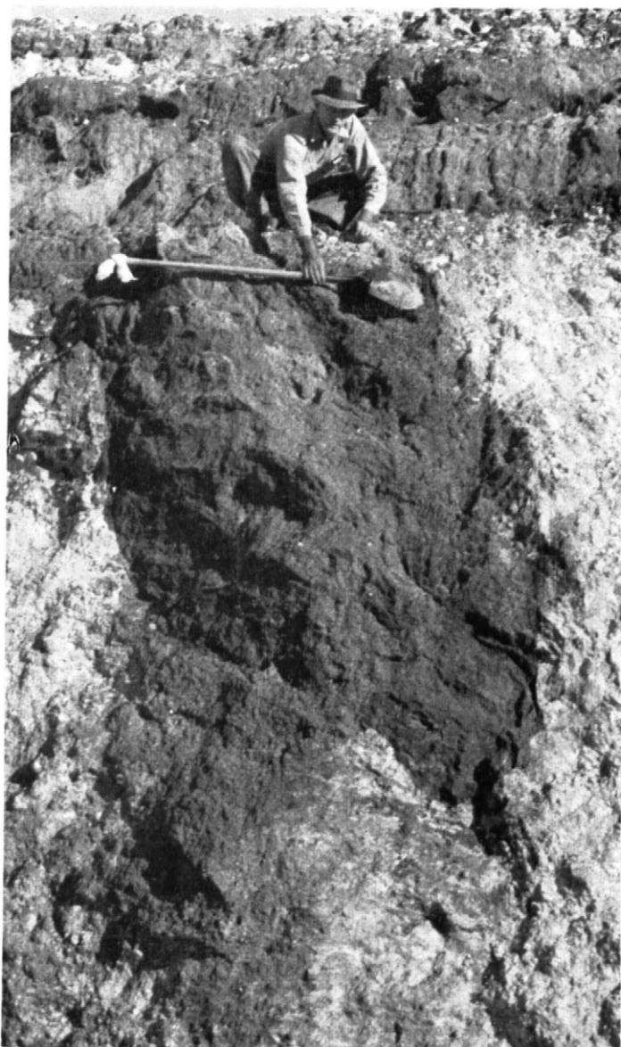
Figure 25. —Solution hole in Suwannee limestone filled with clay from overlying Hawthorn formation. Similar holes, some much larger, are filled with clay or sand from overlying strata and are common in areas of Hernando, Susquehanna, Bowie, and Chiefland soils.
